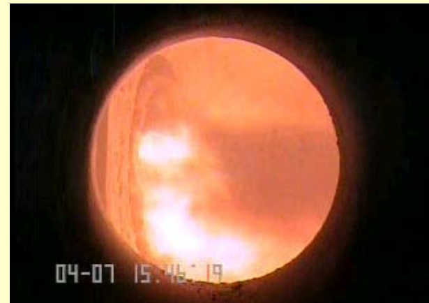
Oxy-Combustion (Pry O 2 =21% ) Photographs of burner flame (4MWth test facility)
