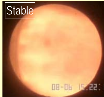
b. Pry O 2 =10%(wet) NR-LE Burner
