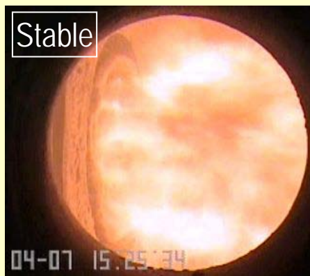
b. Pry O 2 =24%(wet) NR-3 burner
