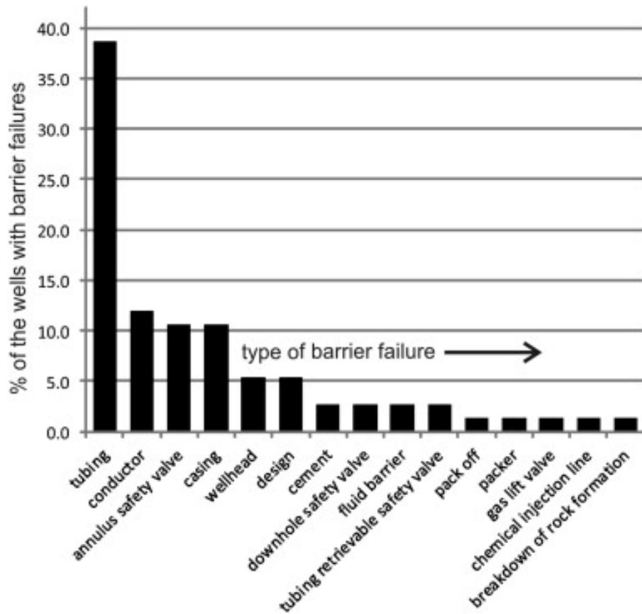
Graph of percentage of well barrier and integrity failures reported in 25 different studies around the world, with drilling dates and number of wells in each study.
