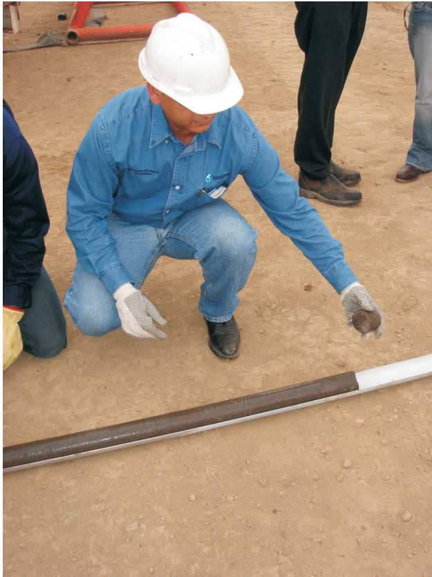
Rock samples are taken by drilling into potential storage sites. These samples show the types of rocks in the formations identified by seismic imaging and they enable the properties of those rocks that affect storage to be evaluated.
