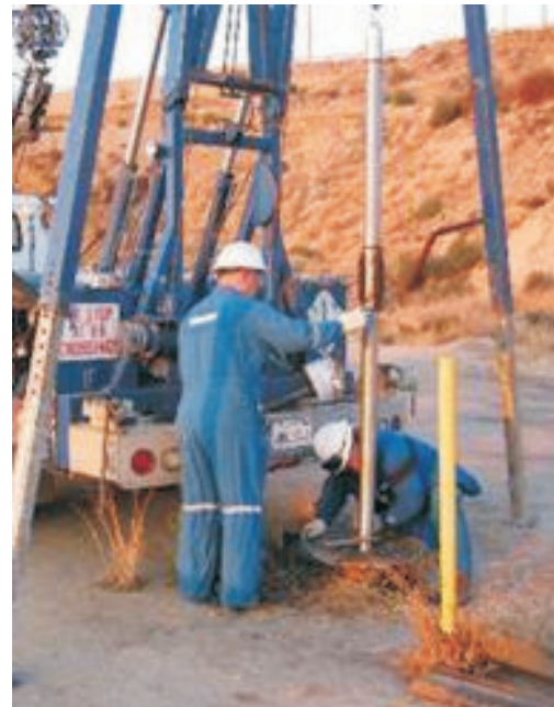
Wireline logs are made by lowering instruments down the well to measure various properties of the rocks along its length.
