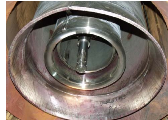
Burner 5: swirl burner with pre-mix possibility
