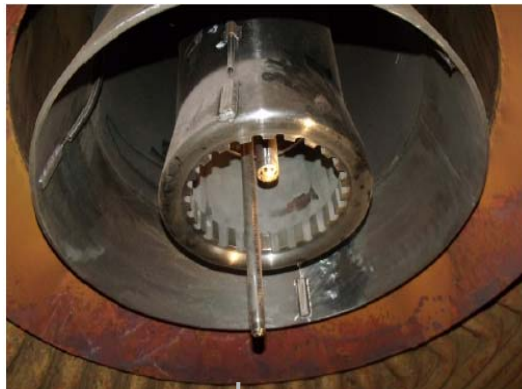
Burner 3: pure swirl burner
