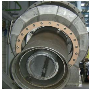
Burner 2: pure swirl burner
